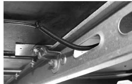
*The pipes must furthermore be protected against sharp edges and corners.*
