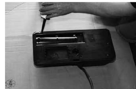
*Bonding the pump housing*
