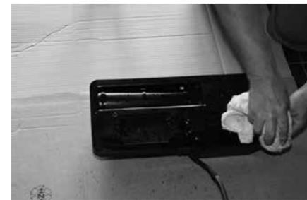
*Degreasing the pump housing*
